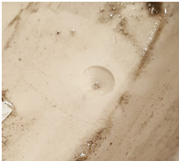
Fig. 12: After six minutes of constant drilling with the masonry bit, we could only penetrate the surface of the porcelain
