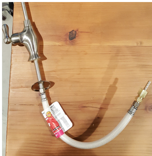
Fig. 8: Refrigerator water line connected to faucet with adapters fitted on the right
