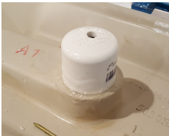
Fig. 11: PVC cap glued to sink drain, before attaching \frac{3}{8} " tubing
