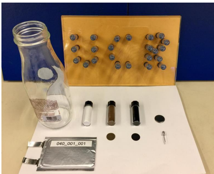
IMAGE: Waste glass bottles are turned into nanosilicon anodes using a low cost chemical process. Credit: UC Riverside
