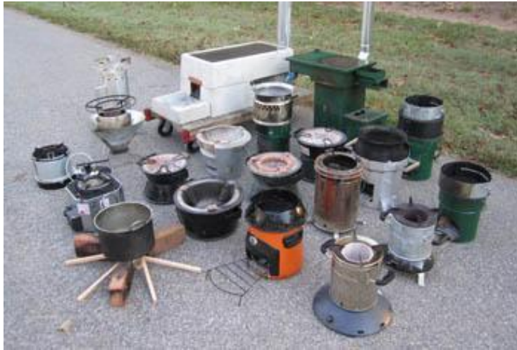
Cookstoves tested for air pollutant emissions and energy efficiency
