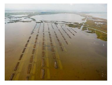
Shoreline protection uses narrow "walls" made of rock or similar materials placed along shorelines of lakes, bayous and open bays. This project type can significantly reduce the rate of erosion of the wetlands and shorelines they protect. Shoreline protection can help maintain existing wetlands as new land is built through marsh creation and sediment diversions.
