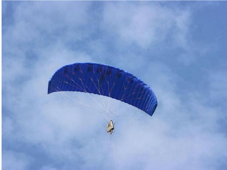
The kite is flown in a figure-of-eight pattern with the tether driving a turbine as it rises Kite Power Solutions Ltd 2015
