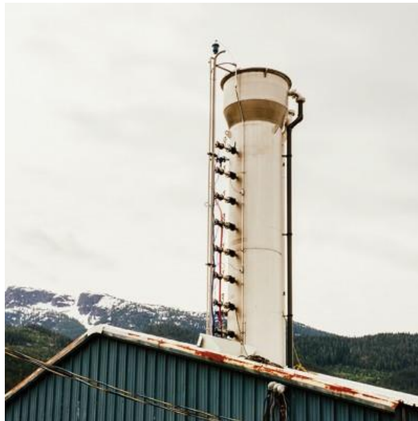
Left: The capture fluid, now rich with carbon dioxide from the air, circulates to a 13-meter-tall reactor. Right: Calcium hydroxide is added to the capture fluid just before it enters the reactor, causing two products to be created inside. One is solid calcium carbonate containing the captured atmospheric carbon. The second, potassium hydroxide, flows back to the air contactor to capture more carbon dioxide.
