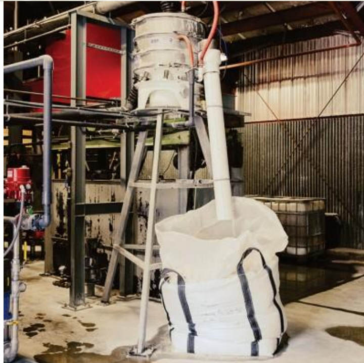
Controlling the formation of calcium carbonate crystals is critical. Fine crystals serve as seeds for future pellets, ensuring the sustainability of the process. Too many fine crystals, however, produce a caustic sludge that's difficult to process.
