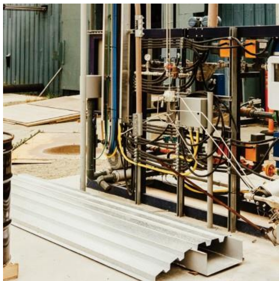
Calcium oxide mixed with water regenerates calcium hydroxide for use in the pellet reactor.
