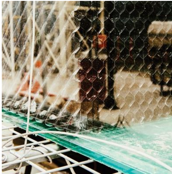
The contactor contains 80 cubic meters of plastic packing whose three-dimensional honeycomb structure offers 16,800 square meters of surface area. The setup removes 75 to 80 percent of the carbon dioxide in the air.
