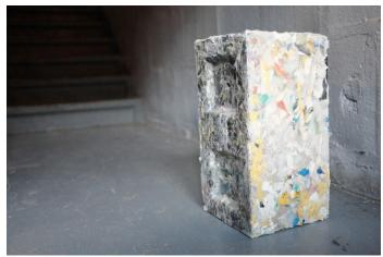
A new startup called ByFusion created an eco-friendly way to repurpose collected ocean plastic permanently, in the form of construction blocks called RePlast.
