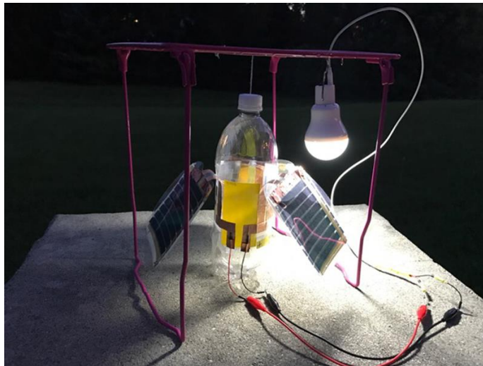
A plastic water bottle at the center provides the structure, and three wings extend off of it. These mimic the leaves on a tree, vibrating in wind or rain, and powering the piezoelectrics. (Discovery Education 3M Young Scientist Challenge)
