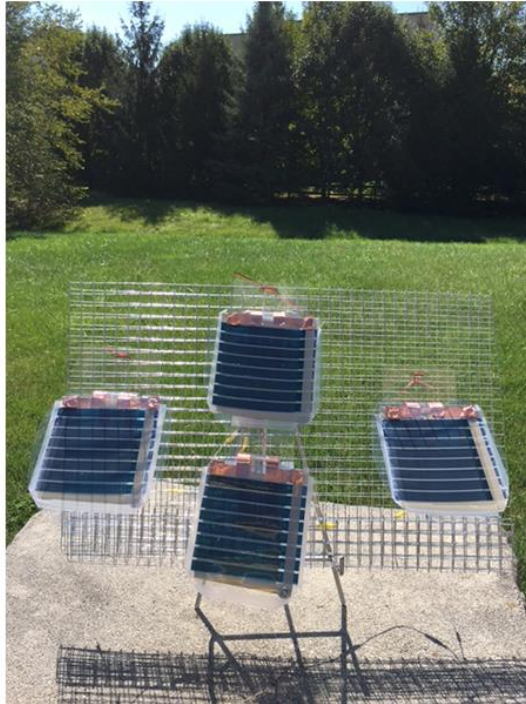
The leaves are made from solar foil, an organic photovoltaic from 3M, which Mendu wired into the same circuit to increase the current. Piezoelectrics are a good source of voltage, but offer little current, and photovoltaics can help supplement that. (Discovery Education 3M Young Scientist Challenge)
