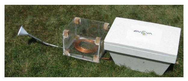
The WindChill fridge uses evaporation to keep food cool. (Photo: WindChill/Biomimicry.org)
