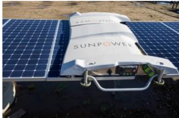
SunPower uses robots to clean solar panels in order to cut water use and lower the labor cost. Photograph: Robert Durrell/The Guardian
