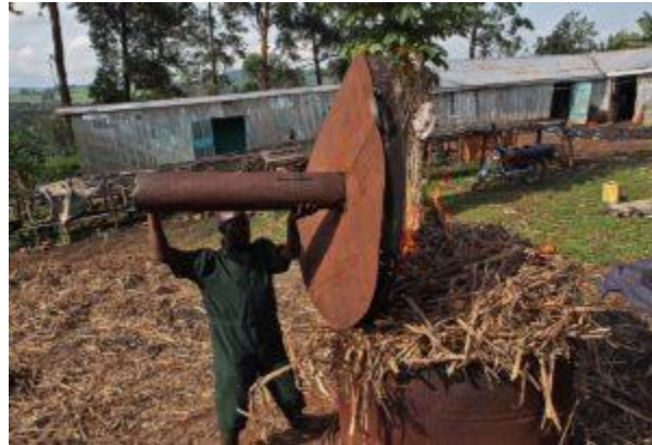
A worker burns sugarcane waste, part of the process in making biochar, at the Eco Fuel Africa factory in Lugazi, Uganda
