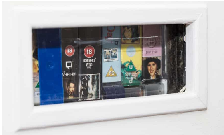
Cassettes being tested for insulation properties. Photograph: University of Brighton
