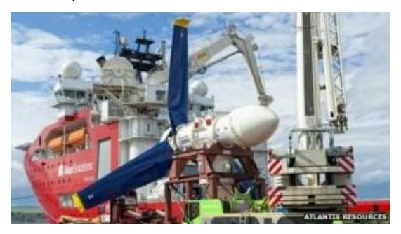
Each of MeyGen's AR1000 turbines stands 22.5m (73ft) tall and weighs 1,500 tonnes
